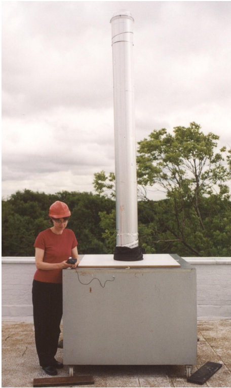
Figure 4 Light pipe under test on roof
